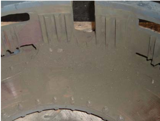
Heavy Brake Dust from counterfeit friction material
