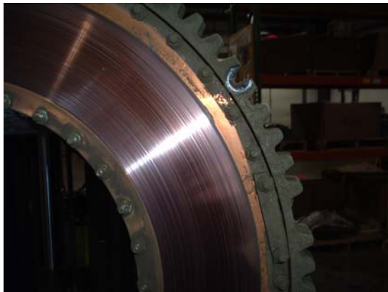
Rapid Copper wear from counterfeit friction material
